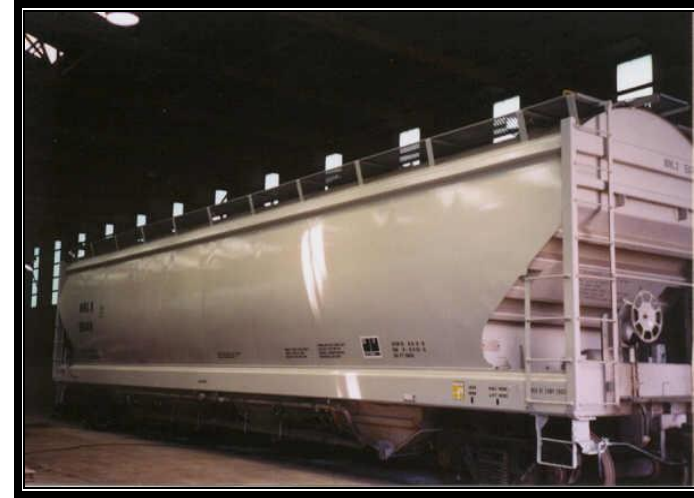
Reconstructed Covered Hopper After Repairs and Painting
